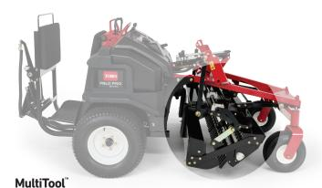
The Field Pro MultiTool is an innovative design that includes an integrated grader and an adjustable tool carrier to quickly and accurately grade, groom and perfect your infields. When fitted with the optional laser grading system the Field Pro 6040 will easily grade your infield for optimal game playing conditions.
